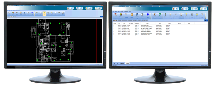
Figure 1: TrueSite Workstations can support Multiple Monitors (touchscreen monitors with expanded desktop shown)
